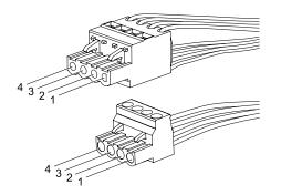
Figure 22.1 CAN Connector Two connectors. 1. 0 V 2. +24 V 3. C1 Signal 4. C2 Signal
