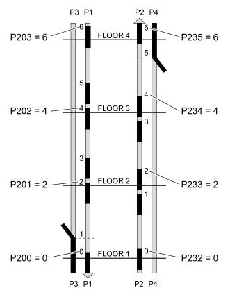
**Figure 9.3 Example Floor Position** The position of the floor is set by entering the number of the flag at the floors parameter. Flag number is entered for both Upward (P2) and Downward (P1) running.
