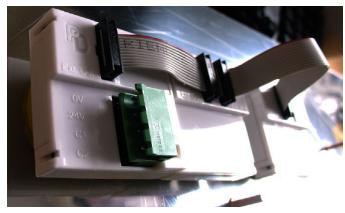
**S4-PB05** is serial-assembled. 7 slave units can be connected to a master unit, which facilitates the installation and reduces the number of connections.
